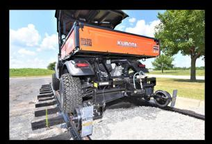
Our optional Composite Rail Wheels have and hardened steel tread with aluminium inner separated by special dialectic neoprene that cuts down on rail head noise up to 95%. The Rail Wheels are naturally insulated.
