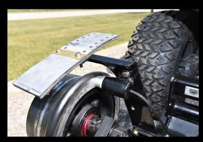
Our Flexiride® Rail Gear has 4 wheel independent suspension that self-compensates for uneven track conditions. The basic system is provided with forged steel rail wheels, a self-contained hydraulic power unit with emergency hand pump, mobile hydraulic valve kit, front and rear rail sweeps, remote control, FRA lights and alarms (stobe not included),plug and play wiring harness, Hose kit, and hydraulic safety locks. (Some assembly required)
